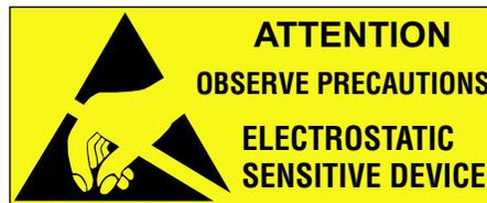
This equipment contains components that may be damaged by “static electricity”, or electrostatic discharge. To prevent this from happening, be sure to follow the guidelines in Adaptive Tech Memo 00-0005, “*Preventing Electrostatic Discharge (ESD) Damage,*” available on our Web site at <http://www.adaptivedisplays.com>.
