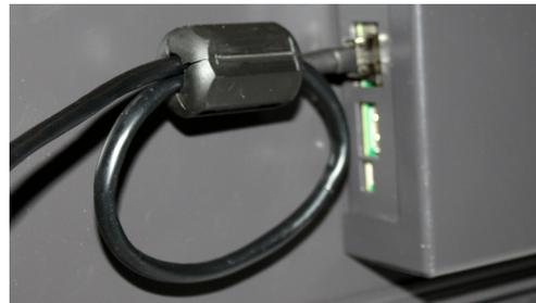
Ferrite installed on Ethernet cable
