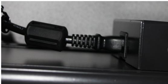
Ferrite installed on power cable
