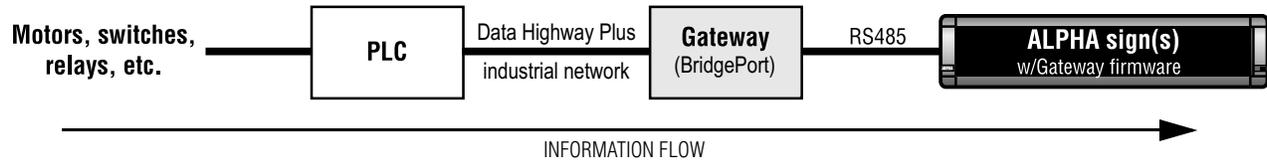
**NOTE:** In the event of a communication failure, caused by any means, messages may not be displayed on a sign.
