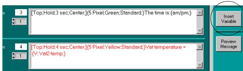
C. Using the scrolling arrows for the Variable Number, scroll through the list of variables available until you locate the correct one. In this case, for Vat2-temp, it is Variable Number 1, therefore the register number is 1.
