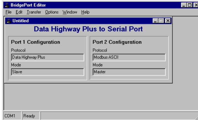
NOTE: If the **BridgePort Configuration Editor** opens with an empty screen instead of with the “Data Highway Plus to Serial Port” window, you must create a new “project” file by selecting *File > New*.
