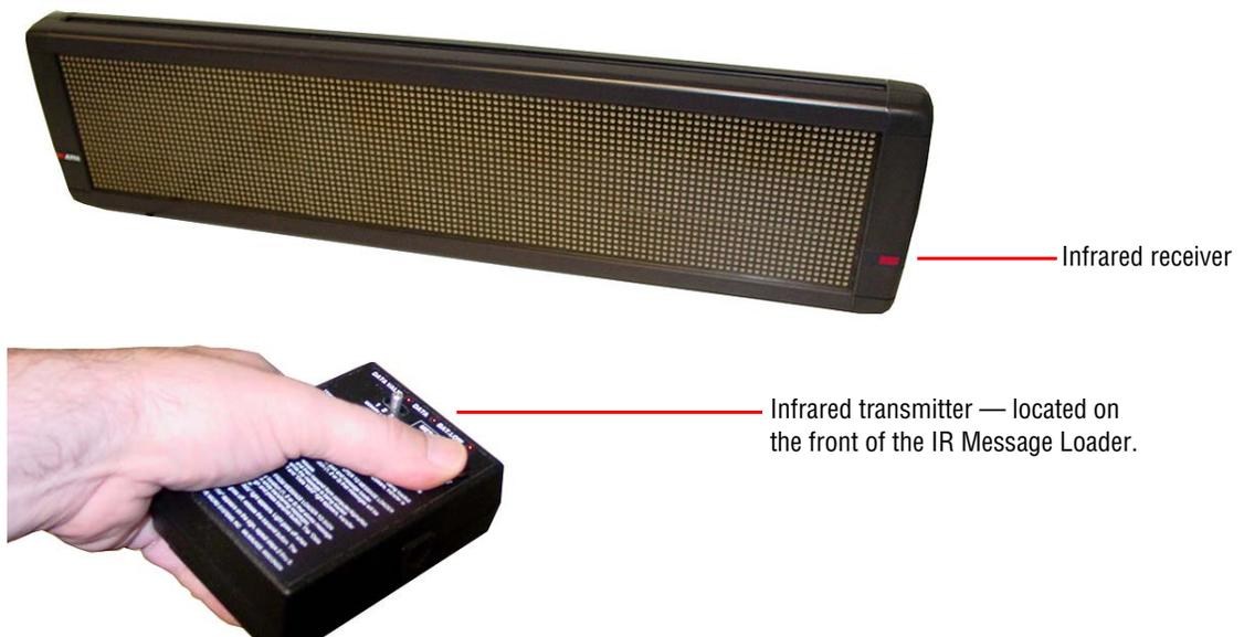
3. Press and hold *TRANSMIT* on the IR Message Loader. Watch the *DATA* light. When it goes off, stop pressing *TRANSMIT*.
