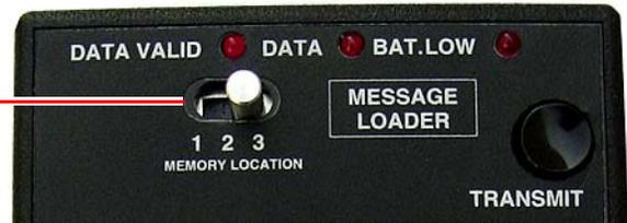
2. Press and release *TRANSMIT* on the IR Message Loader. When *DATA* blinks once, go to the next step. You only have 10 seconds.
