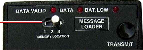
4. On the IR Message Loader, press and hold *TRANSMIT*. Watch the *DATA* light. When it goes off, stop pressing *TRANSMIT*.
