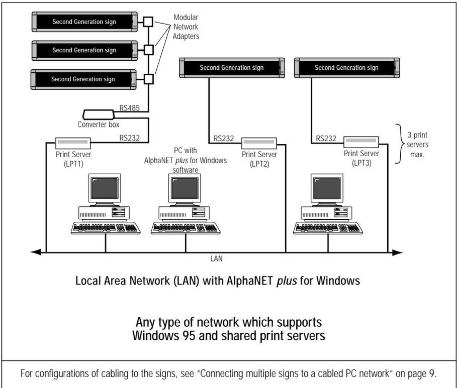
This method of connecting signs allows you to use any existing LAN network software that can support connecting LPT ports to a print server. Examples of this type of network software are Windows NT server, Windows 95 peer-to-peer, Novell, Banyan Vines, etc. However, on this network, each PC with AlphaNet *plus* for Windows can only be running Windows 95 operating system software. Windows NT is not supported on PCs with AlphaNet *plus* for Windows and print servers.
