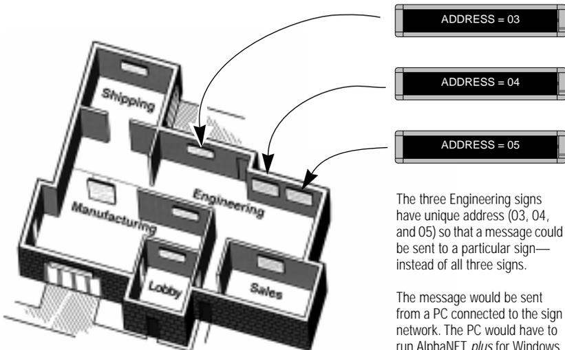
The three Engineering signs have unique address (03, 04, and 05) so that a message could be sent to a particular sign—instead of all three signs.
