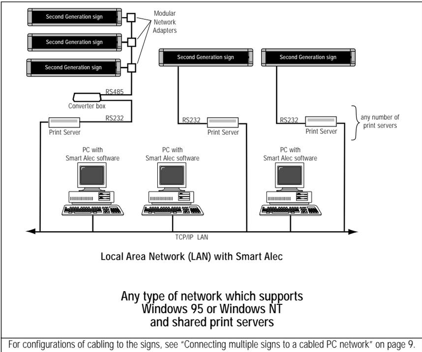
This method of connecting signs allows you to use any existing LAN network software that can support TCP/IP. However, on this network, each PC with Smart Alec can only be running either Windows 95 or Windows NT operating system software. Smart Alec is designed to be networking software, so it can be installed on any number of computers in the network.
