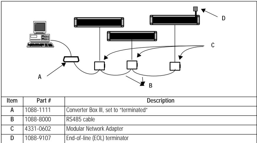
Table 31: The right way to connect ALPHA signs at a Converter Box with *two* sign cables
