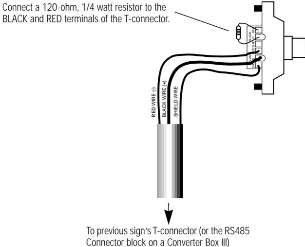
Figure 2: Terminating an Older Generation sign
