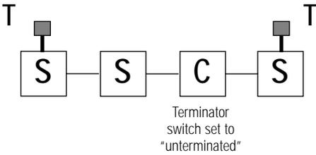
Figure 4: End-of-line termination
