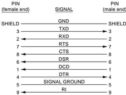
*10 foot, 25 pin-to-9 pin, type "B9" RS232 cable (1088-8635)*
