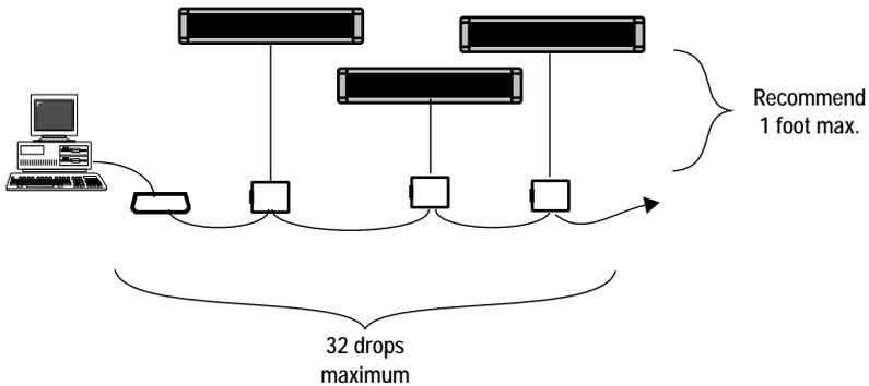
Figure 1: Maximum network drops and cable length
