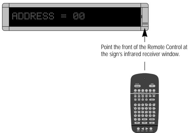
3. Press the **PROGRAM** button on the Remote Control. The words PROG TEXT FILE A will appear on the sign.
