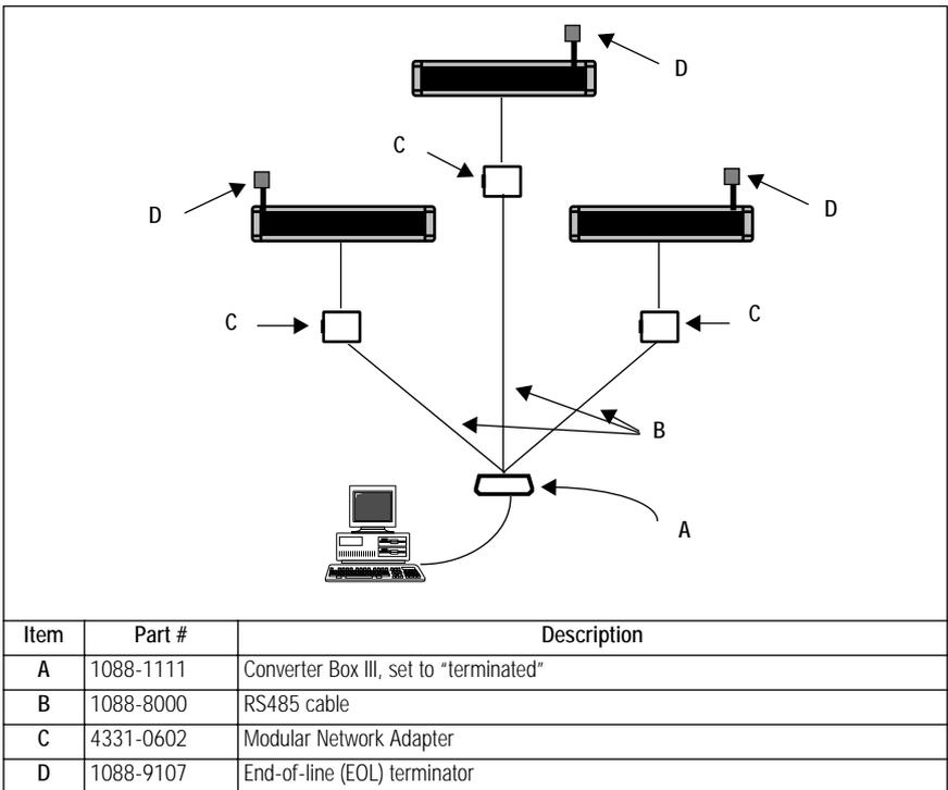
The right way to connect ALPHA signs at a Converter Box has only one or two sign cables coming out of the Converter Box. This works well because the signs are “daisy-chained” so the electrical load at the Converter Box is minimized.
