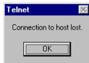
13. After clicking *OK*, and after the serial server completes rebooting, you can connect to the server using the new IP address if you wish to confirm the change with the **show server** command. Alternatively, you can exit **Telnet** and send messages.
