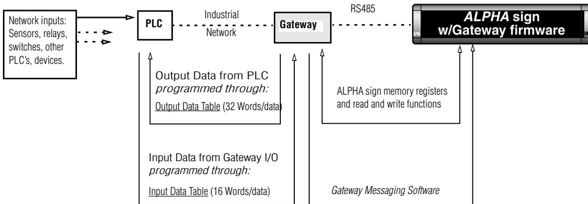
**INFORMATION FLOW**—In a Profibus DP network, a “device” is any point in the information pathway that is capable of sending or receiving a data signal. In the most basic network configuration, above (one input, one PLC, one Gateway interface, one sign), the PLC, Gateway interface, and sign are all capable of both sending and receiving data signals.
