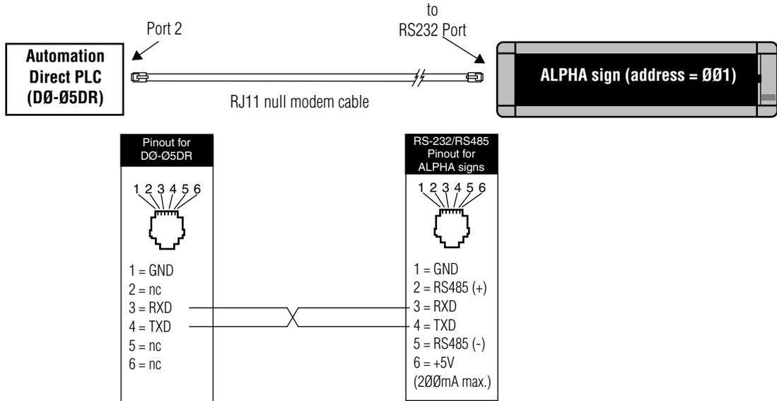
Figure 2: Connecting an Automation Direct PLC to *one* ALPHA sign using a null modem cable
