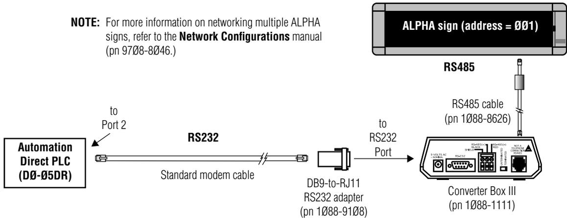
Figure 3: Connecting an Automation Direct PLC to *more than one* ALPHA sign using a standard modem cable
