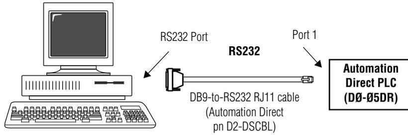
**Figure 1: Connecting a computer to an Automation Direct PLC**
