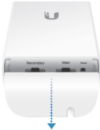
2. Connect the molded end of the Ubiquiti PoE Outdoor Adapter (P/N 12883100) to the *LAN* port.
