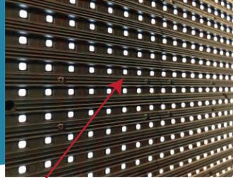
Advanced and almost unbreakable stepped louver design that displaces light and provides better contrast
